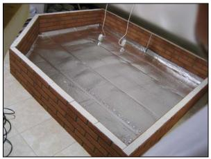
A layer of insulating foil thermally isolates the soil substrate from the concrete floor. For aesthetic reasons, the Ytong blocks were covered with artificial (light-weight) stone strips.
